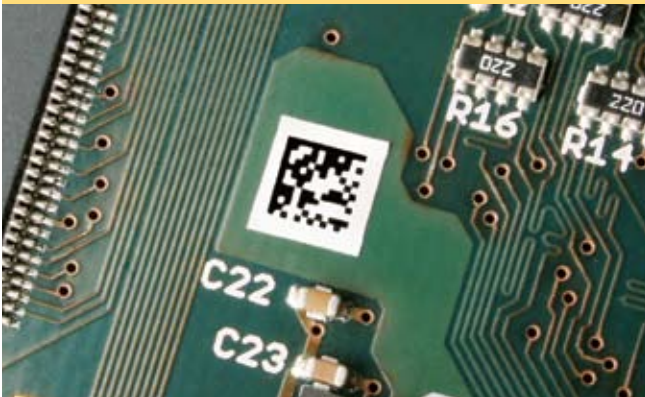
Smallest label size of 4 x 4 mm, if there is only little space.
